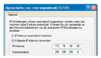
The PC's and the R&S ETH's subnet mask must also match in order to make a connection.
