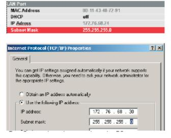
Select the SUBNET MASK menu item from the list below the heading LAN PORT with the rotary knob or the cursor keys (Λ or V) and confirm with ENTER. An input field opens.  Enter the subnet mask used on the PC, e.g. 255.255.255.0 with the numeric keys and confirm with ENTER.
